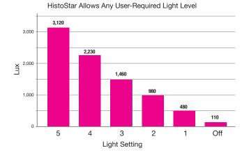
Figure 2. Specimen area luminance at each setting.
