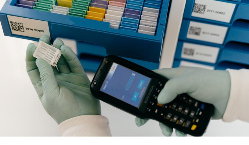
In just minutes, the Arcos system scans hundreds of blocks and records their exact location — from the position in the tray to the final storage point (zone) in a laboratory's on or offsite archive. The system is designed to help reduce the risk of losing blocks, improve operational efficiency and expand workflow capacity for both short and long-term storage.
